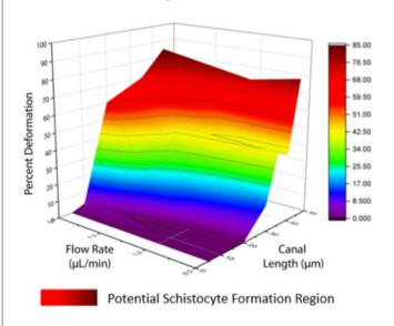
Figure 5. 3D graph of percent plastic deformation of erythrocytes (z-axis and color spectrum) as a function of canal lengths in  $\mu$ m (x-axis) and flow rate in  $\mu$ L/min (y-axis). Flowrate is directly related to shear rate (s<sup>-1</sup>).
