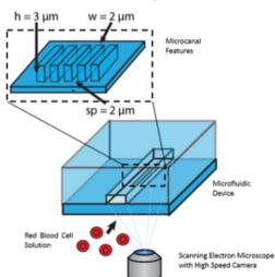
Figure 3. Model of experimental microfluidic system. Each device is comprised of five columns that form "microcanals" that are 2  $\mu$ m wide and 3  $\mu$ m tall with lengths varying between 5  $\mu$ m and 45  $\mu$ m.
